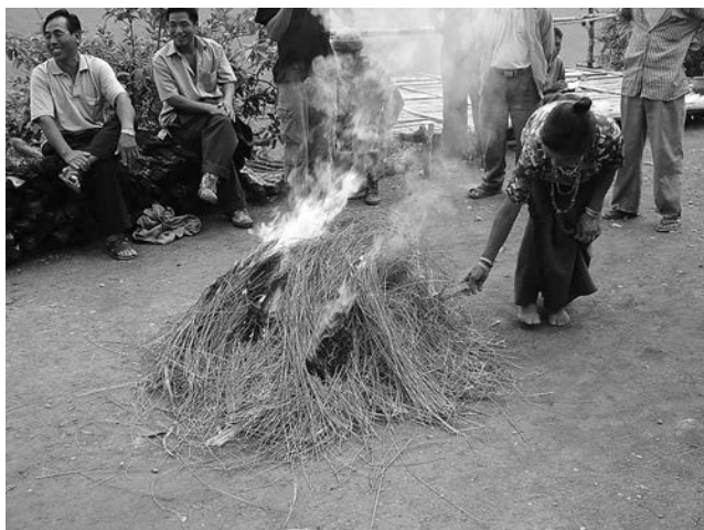
Fig. 14: Firing pots by covering with firewood and grass (Photo by A. Aier)
