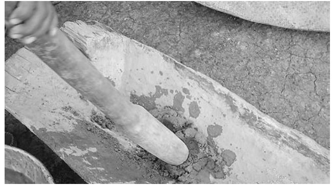
Fig. 4: Re-pounding of clay to increase plasticity
