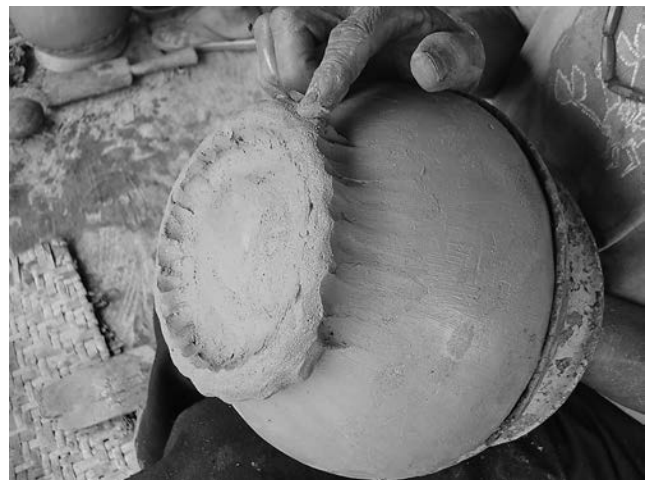
Fig. 8: Fusing the ring to the base (Photo by A. Aier)
