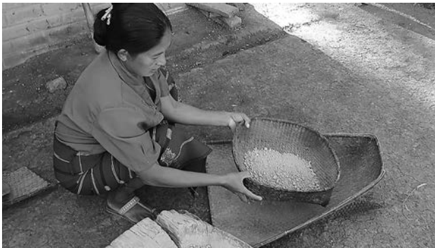
Fig. 3: Sieving the pounded clay
